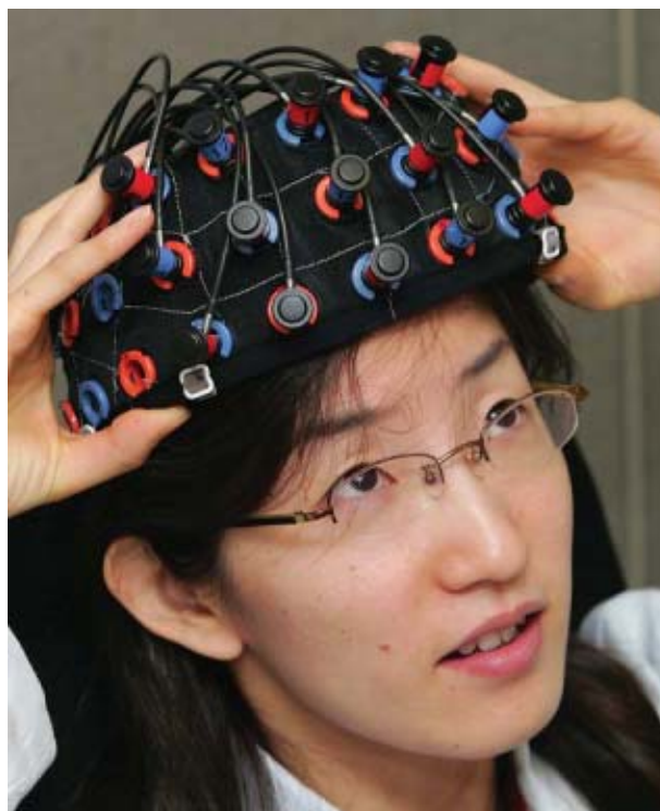
Developed by Hitachi, this brain-machine interface analyzes slight changes in the brain's blood flow and translates them into electric signals, allowing the device's user to control everyday objects without lifting a finger.
